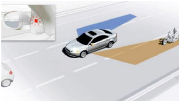
Figure 2: Blind spot detection
