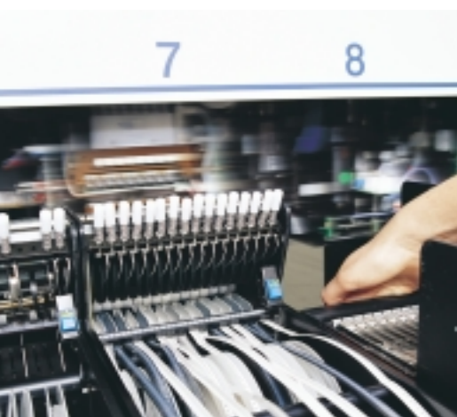
Removal and refill of feeders is possible while the machine is placing components. If a magazine runs out of one component, production doesn't stop. Instead, the machine alerts the operator, re-optimizes and continues to mount the remaining components.
